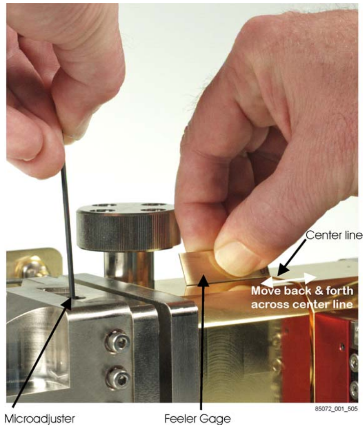
Figure 5-5 Using the Feeler Gage
