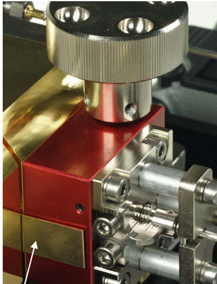
Feeler gage inserted from front of resonator at center line of gap between cylinder halves
